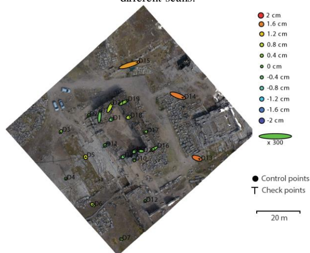
Figure 16. Spatial distributions of residual on GCPs and CPs (under 0.01 meters on the building and up to 0.015 in surroundings)
