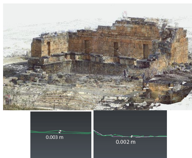
Figure 15. The final overall points cloud (25 ml points) and (below) very low distances among profiles extracted from different scans.
