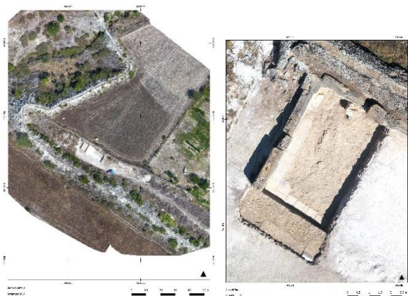
Figure 9. (left) 0.017 m per pixel orthophoto showing the two parallel channels flowing to north. (right) the 0.004 m resolution orthophoto of the basin.
