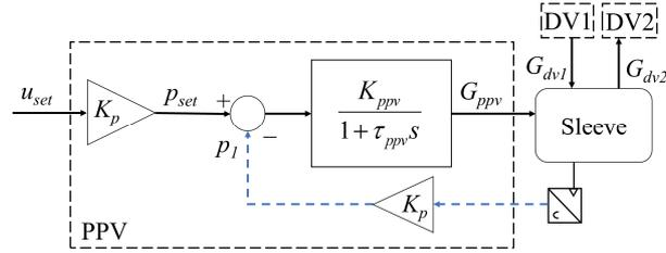
**Fig. 3.** Model of the pressure proportional valve.
