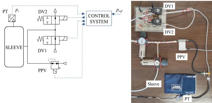
**Fig. 1.** The pneumatic system for hyperemia stimulation: DV1 - 2/2 digital solenoid valve for sleeve supply; DV2 - 2/2 digital solenoid valve for sleeve discharge; PPV - pressure proportional valve; PT - pressure transducer.
