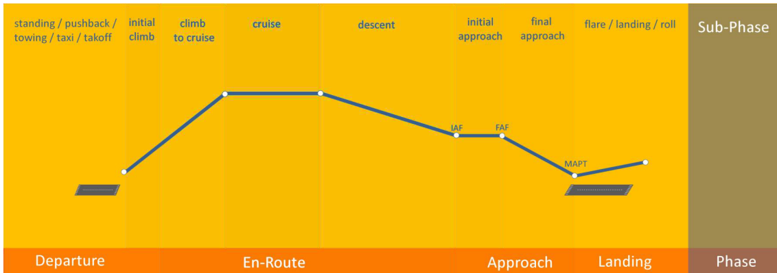
Figure 2.1: Typical phases of flight [87]
