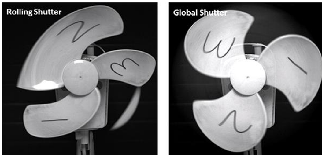
Figure 1.9: Example of distortion generated by the rolling shutter readout (on the left) and the same picture obtained with a global shutter (on the right)
