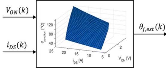
Fig. 4: Functional block for the online temperature measurement
