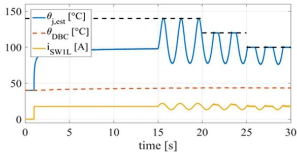
Fig. 5: Estimation and limitation of the junction temperature.
