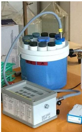
**Fig 4.1 Pulse-amplituted modulated (PAM) and filtration system .**
