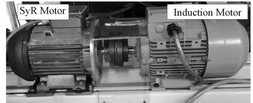
Fig. 15. Synchronous reluctance motor coupled with an induction machine.
