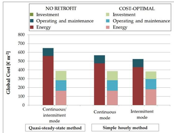
Fig. 3 – Global cost, no retrofit and cost-optimal solutions
