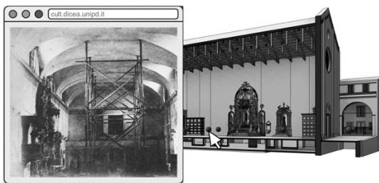
Figure 3. All the instances in the model are linked with the object in the database. The image shows an example of integration of historical photos in the BIM: spherical entities with an URL link refer to the images and allow to visualize them in real time.
