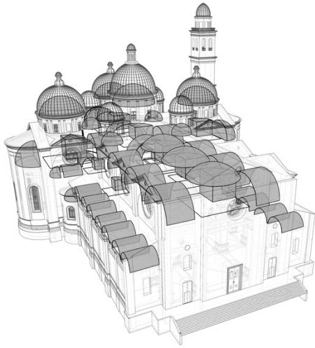
Figure 5. Exploiting the potential of the BIM tool an interesting cataloguing of parametric objects has been created, they are virtual entities of the structural stubs and have been used as a “negative” surface to realize the vaults and domes.
