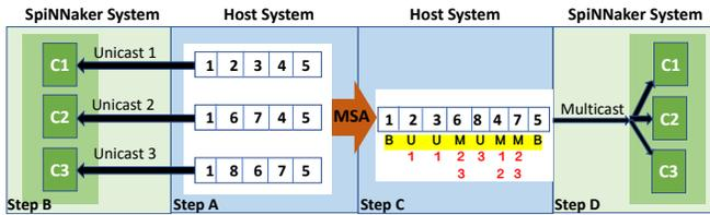
Fig. 2: Dataflow for current and MSA implementations
