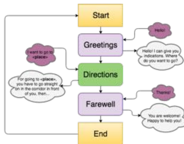
Figure 5. Robotic receptionist's conversation logic.
