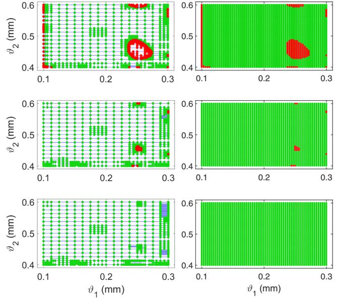
Fig. 1. Identification of regions  $\Theta_q \subseteq \Theta$  where at least one imaginary Hamiltonian eigenvalue exists (red dots: non-passive, green dots: passive). Left panels: results of proposed adaptive sampling scheme. Right panels: validation through a fine uniformly sampled grid. The three rows correspond to the passivity checks of three different iterations of a passivity enforcement scheme applied to a PCB interconnect macromodel.
