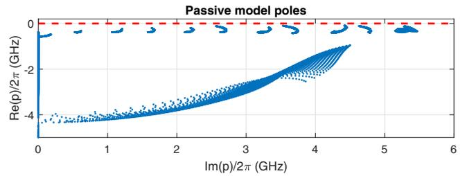
Fig. 3. Superposition of all poles computed for the PCB link parameterized model, instantiated at a finely sampled grid in the parameter space.
