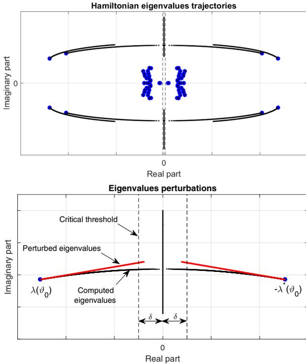
Fig. 2. Hamiltonian eigenvalues. Blue dots: eigenvalues  $\lambda_i(\vartheta_0)$  at a fixed parameter value  $\vartheta_0$ . Black lines: exact eigenvalue trajectories  $\lambda_i(\vartheta)$  for  $\vartheta = \vartheta_0 + \Delta\vartheta$ . Red lines: approximate eigenvalue trajectories  $\tilde{\lambda}_i(\vartheta)$  based on linear perturbation theory.
