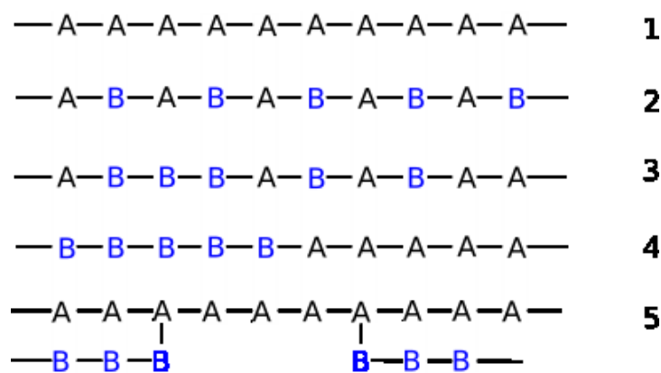
Figure 2.2 - Arrangement of copolymers repeating unit: (18.1) homopolymer (18.2) alternating copolymers (18.3) random copolymers (18.4) Block copolymers (18.5) grafted copolymers
