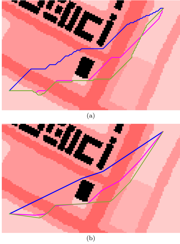
Fig. 9 Path planning with A* (in blue), RA* (in magenta) and riskA* (in green). In (a) only the path planning algorithm is executed, while in (b) the Post-Optimization procedure improves the path.
