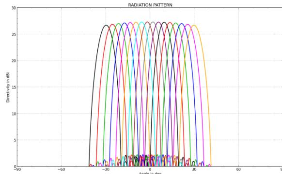
Figure 5: Simulated directivity of the antenna array driven by the Rotman lens without employing the new concept.
