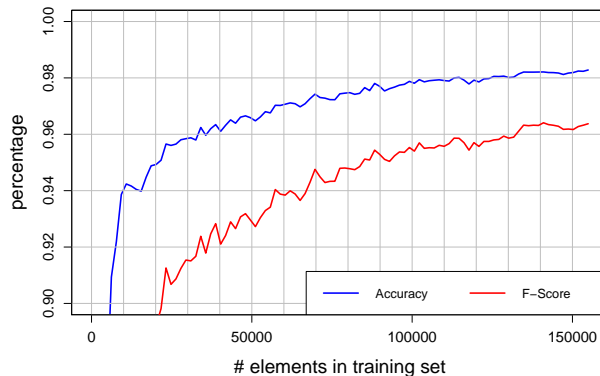
Fig. 10. Accuracy and F-score of the decision tree algorithm versus the number of points used in the training set.
