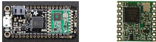
FIG. 1 – Adafruit® Feather 32u4 LoRa Radio RFM9 on the left and LoRa Radio RFM9 transceiver module on the right.
