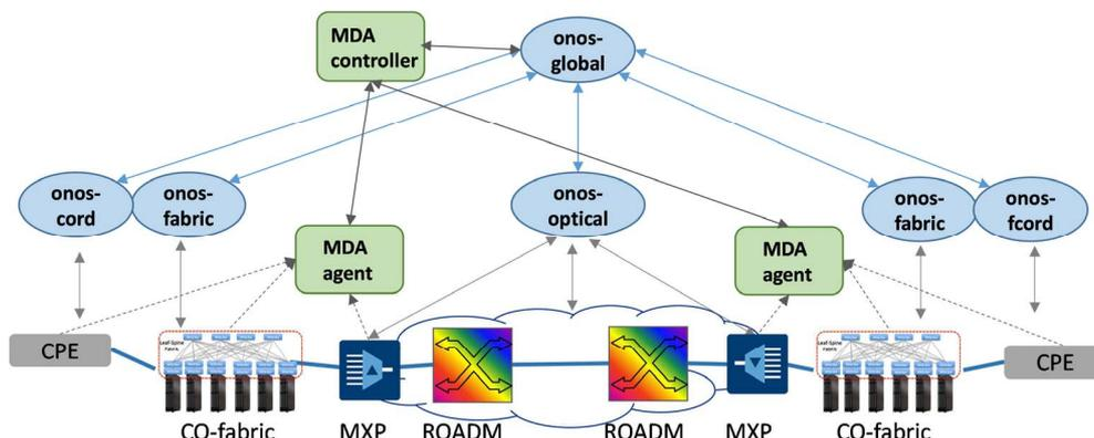
Fig. 1: Network controllers view and monitoring architecture
