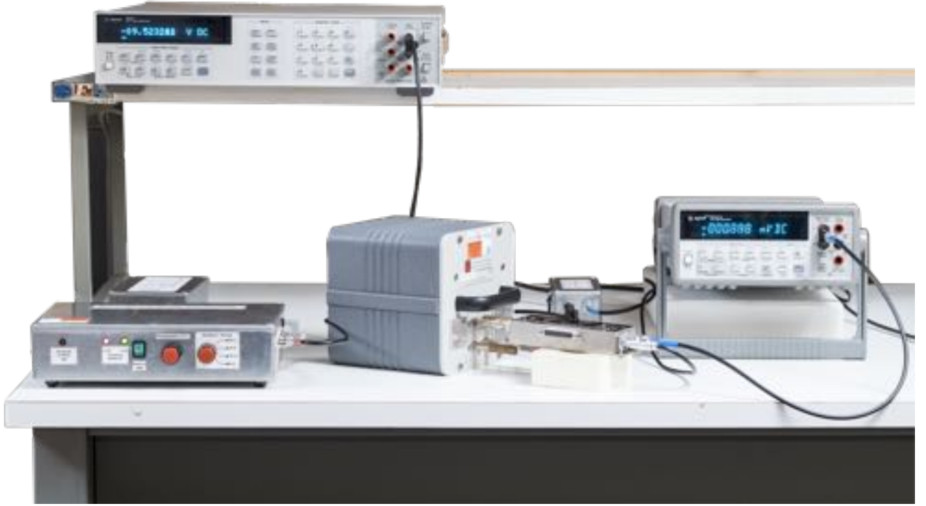
Fig. 3. A photo of the calibration setup corresponding to the schematic diagram of Fig. 2. The source G (for the dc current calibration mode) is on the bottom left; C and A in the center; V_{in} on top left; V_{out} on the right. A detail of C and A is given in Fig. 4.
