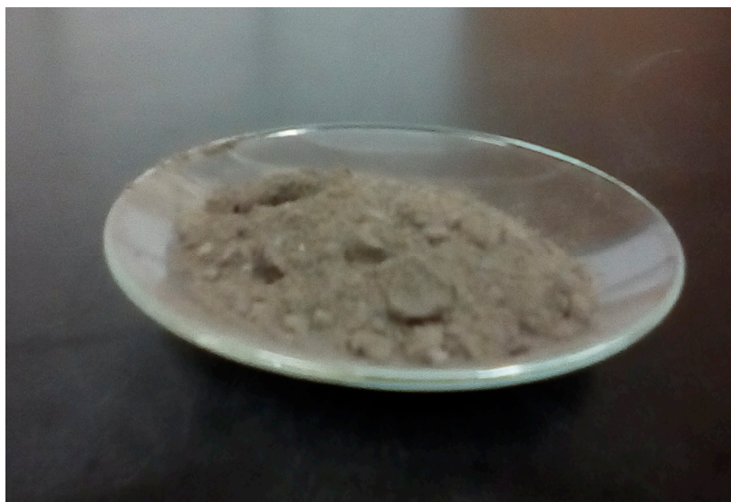
Figure 2. Biosolids-based catalyst as recovered from hydrolysis of biosolid at 280 °C for 1 h.
