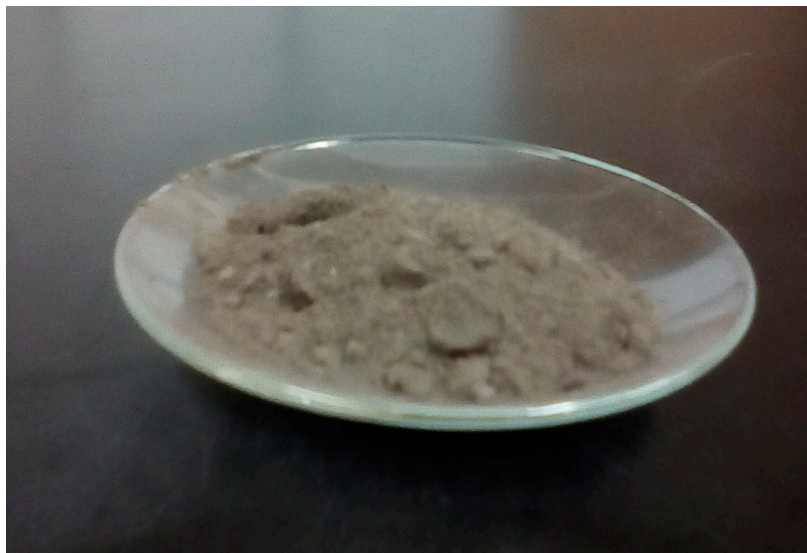
Figure 2. Biosolids-based catalyst as recovered from hydrolysis of biosolid at 280 °C for 1 h.
