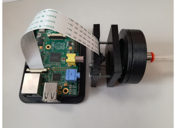
Fig. 2. The prototype of the realized measuring system. In the picture are visible: the RaspberryPI 3 used for image processing, the Raspberry PI Camera 2 module and the collection chamber with a disc filter mounted on. The plastic tube connected to the air pump is also visible at the backside of the collection chamber.
