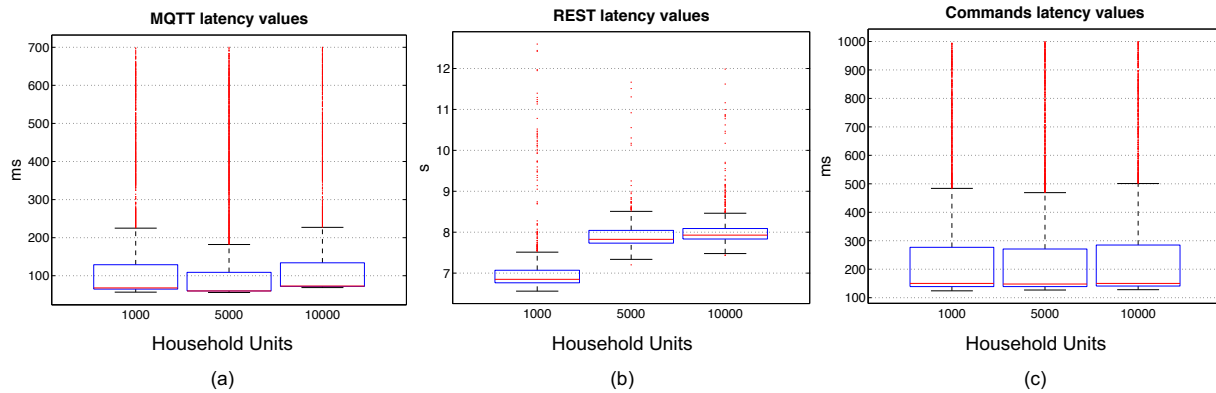
Fig. 11. Transmission latency at different Household Units: (a) MQTT, (b) REST, (c) Commands.
