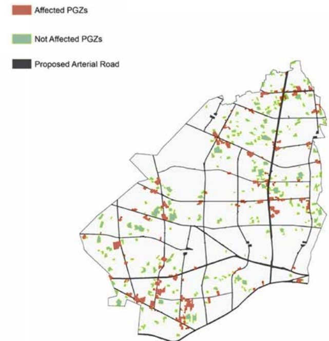
Fig. 3. Affected PGZs by constructing proposed arterial roads.
