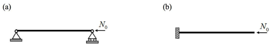
Figure 5. Load and boundary conditions: (a) simply supported beam and (b) cantilever beam under axial compressive force.
