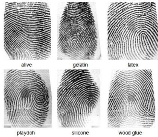
Fig. 2.2 Examples of live and fake samples (created with different materials) from the LivDet 2011 datasets.
