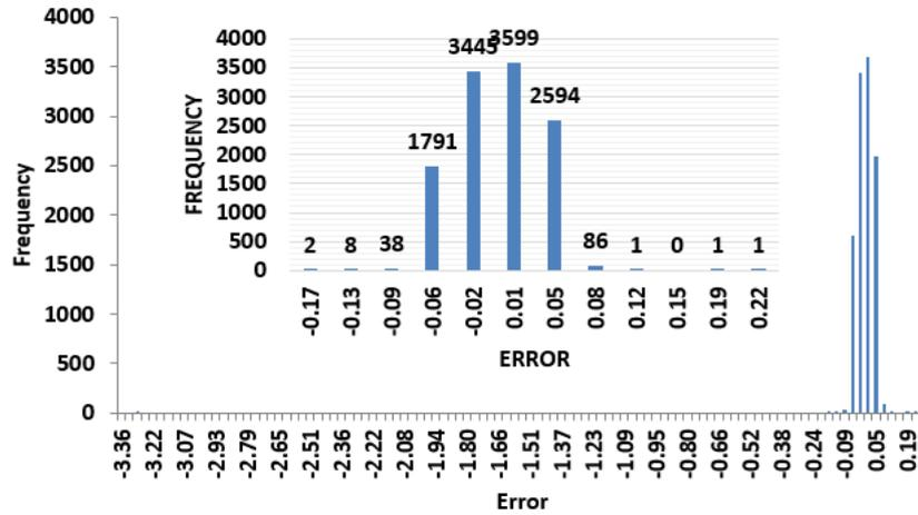
Figure 6.27: Histogram of the error for mean tensile stress on the blade (standard deviation = 0.046).
