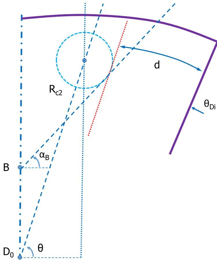
Figure B.4: Disc neck length calculation.
