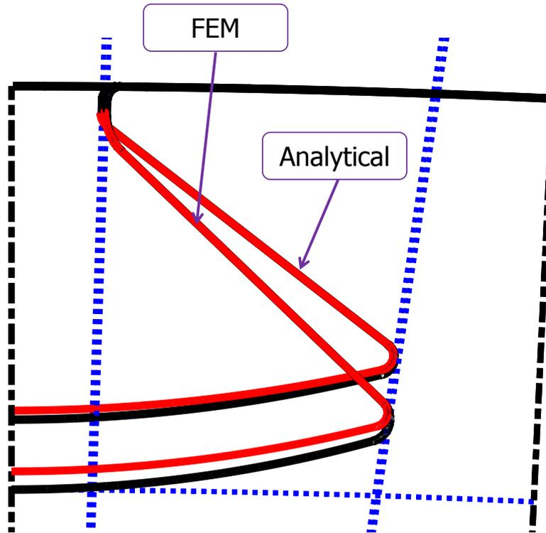
Figure 6.1: the analytical optimum vs. FEM optimum geometry.
