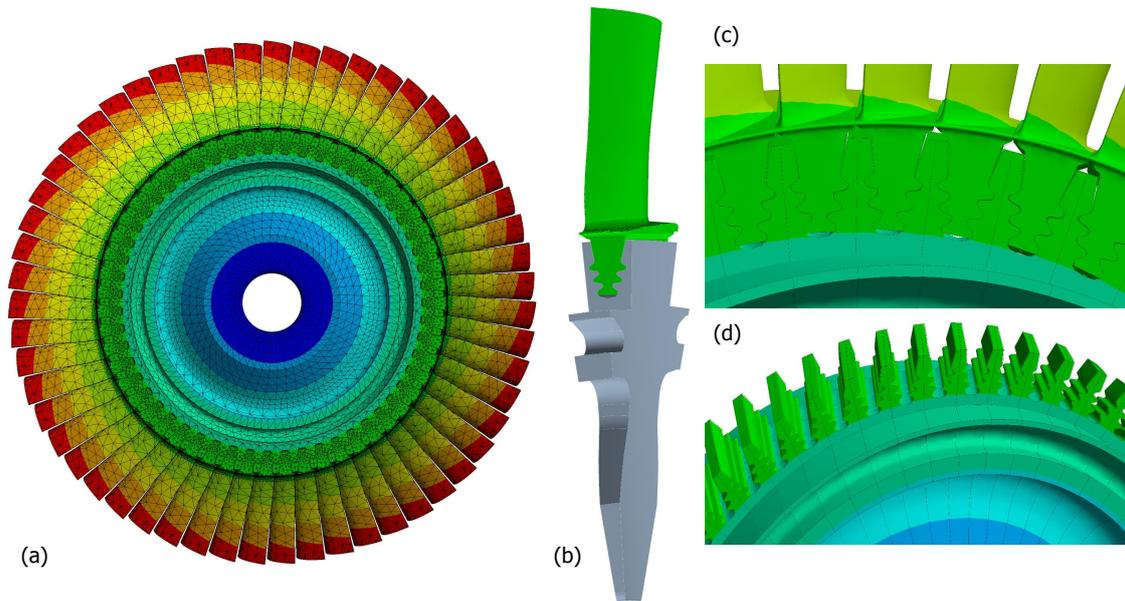
Figure 1.1: Blade and disc typical fir-tree attachment. a) Full disc and blades, b) Blade and its corresponding disc section, c) Close view of the fir-tree attachment, d) Fir-tree groove on the disc.
