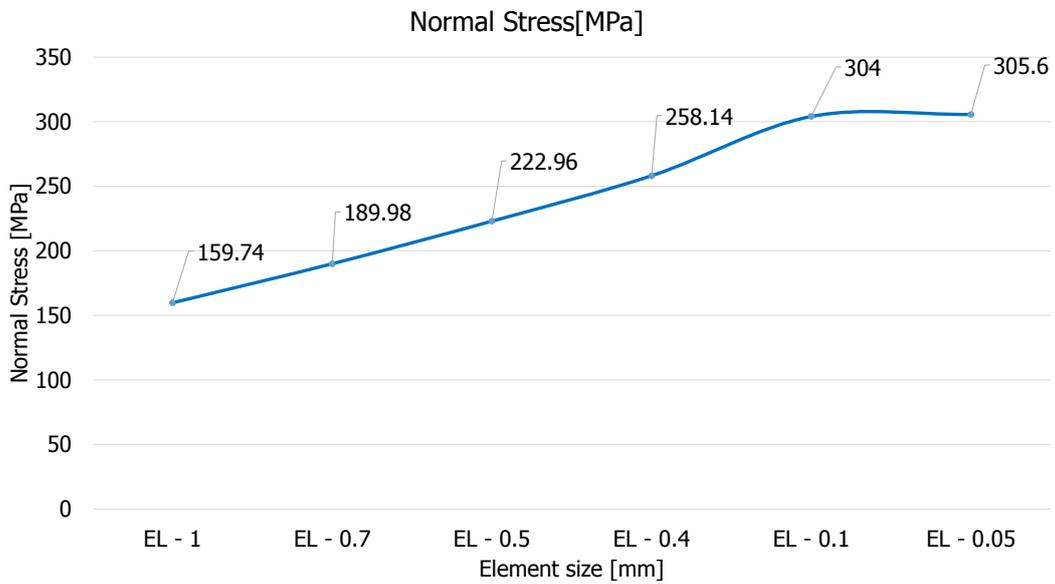
Figure 6.8: Mesh convergence for normal contact stress.
