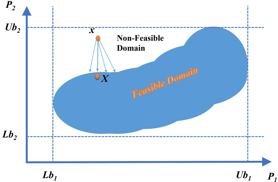
Figure 4.9: Non-feasibility handling by proximity to the boundary of feasible space
