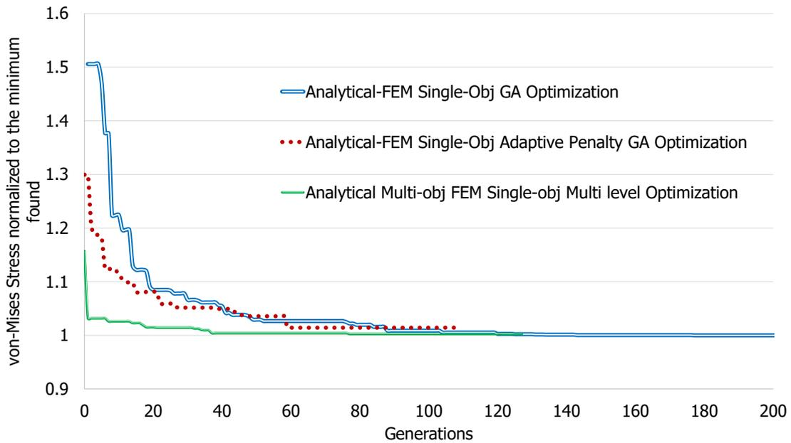
Figure 6.31: The comparison of optimization convergence for different methods.
