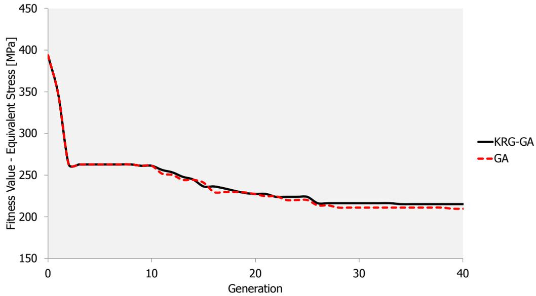
Figure 6.14: Genetic algorithm (dashed line) vs. Co-KRG convergence.
