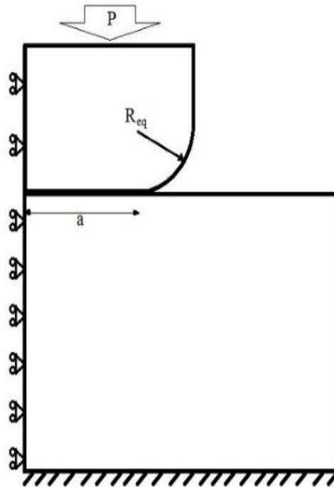
Figure 6.5: Schematics of the equivalent punch test.
