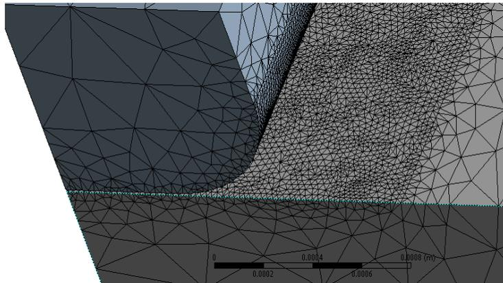
Figure 3.4: Punch 3D FE model mesh density in contact surfaces.
