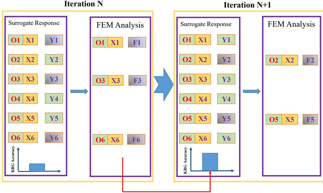
Figure 4.5: Maturation of Kriging Model in every loop.
