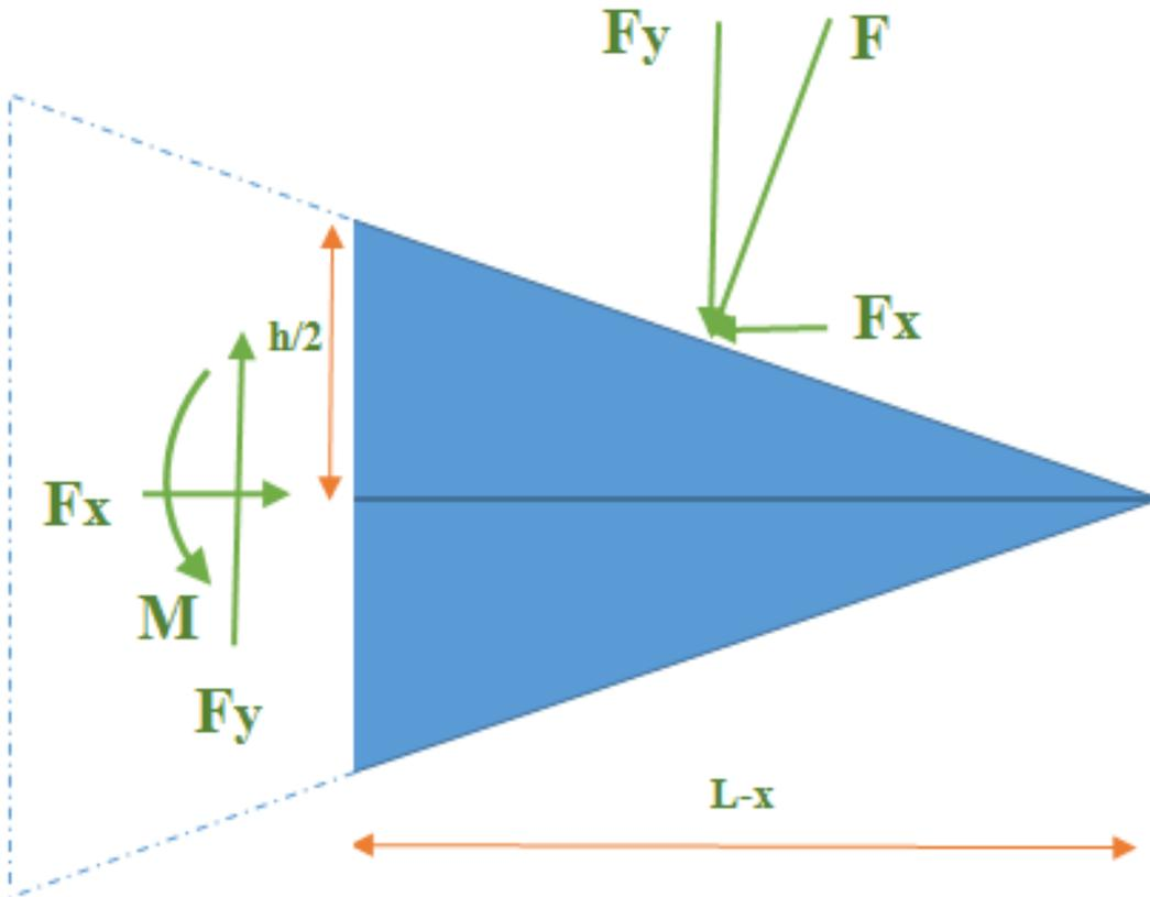
Figure B.7: Free body diagram of a single lob.
