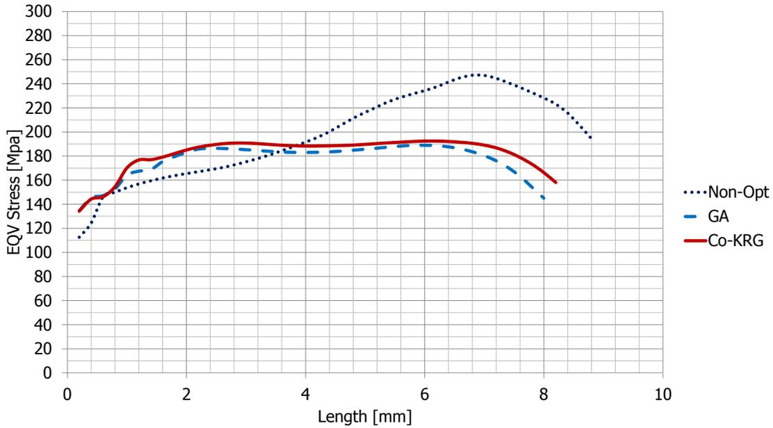
Figure 6.16: Equivalent stress along disc fillet edge.
