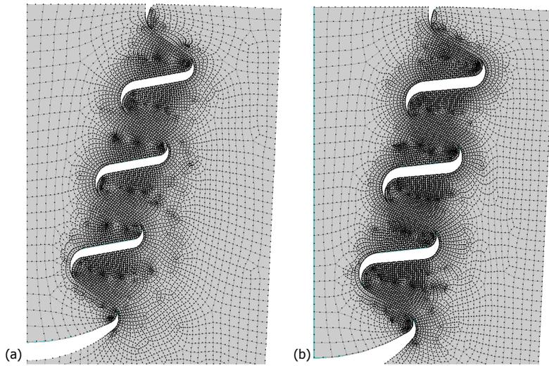
Figure 2.4: Mesh density for two random fir-tree shapes
