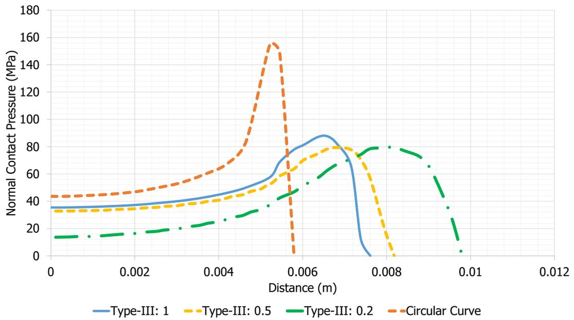
Figure 5.6: Normal Contact Pressure for different Punch Profiles.
