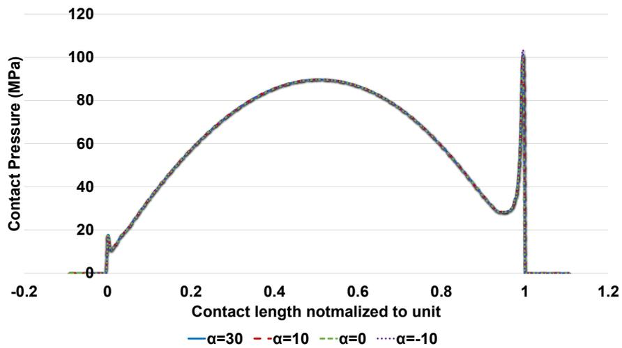
Figure 5.9: contact pressure of polynomial curve (Type-III) joint with different  $\alpha$
