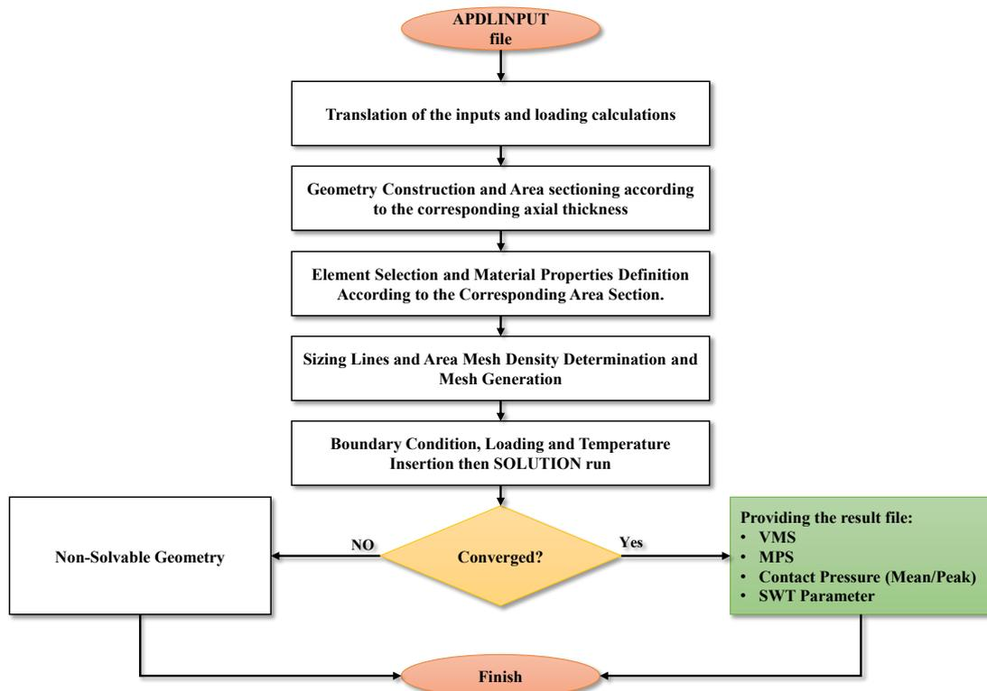
Figure C.3: APDL Batch FE Analysis Flow Chart.
