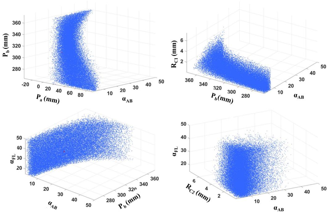
Figure 4.7: Cloud of Feasible space inside the working domain. As the working domain is in a higher dimension than 3D, different illustrations with a different selection of input variable parameters have been shown here (Please refer to Table A.1 for parameters description).
