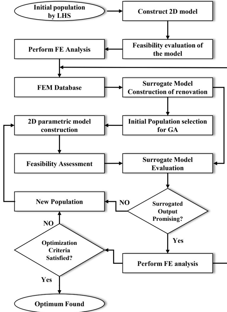
Figure 4.4: Embedding Kriging function into GA optimization.
