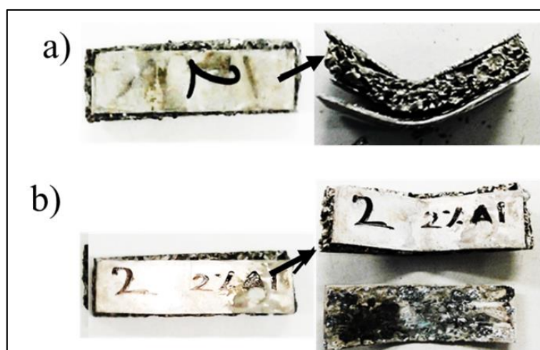
Figure 3-23 Solution heat treated a) AFS-E and b) AFS-F specimens before and after the three-point bending test.
