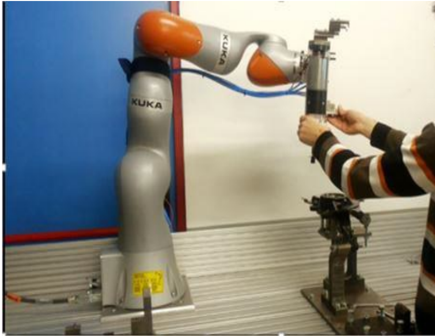
Figure 5.31. Human-robot collaboration with the hand-guided (HG) method during the assembly process of a brake disc.
