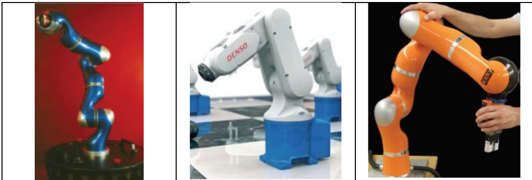
Figure 2.21. Light weighted Arm design: a) KUKA, b) DENSO, c) DLRIII
