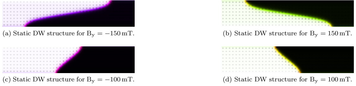
Figure 3.15: Snapshots of DW static structure determined by micromagnetic simulations under static conditions.
