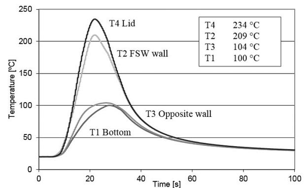
Figure 5. Temperature development during FSW and peak temperatures.
