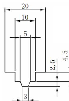
Figure 2. The FSW-tool geometry and dimension (Unit: mm).
