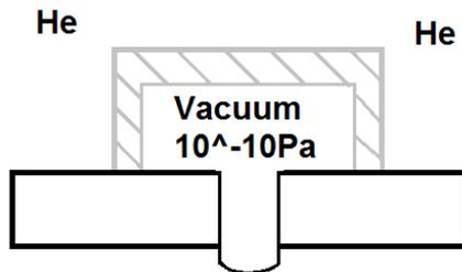
Figure 14. Gas tightness test for half box.
