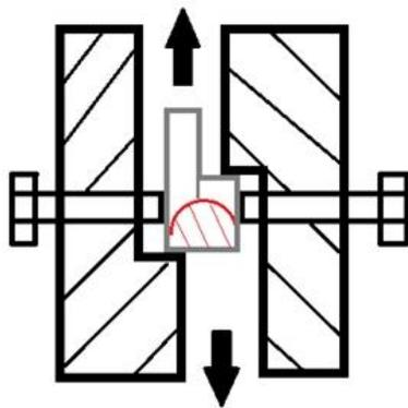
Figure 7. The shear test of FSW specimen.
