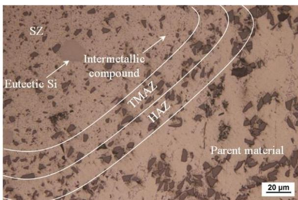
Figure 11. Microstructure of FSW joint of 15 vol% SiC<sub>p</sub>/Al-MMCs with four zones.
