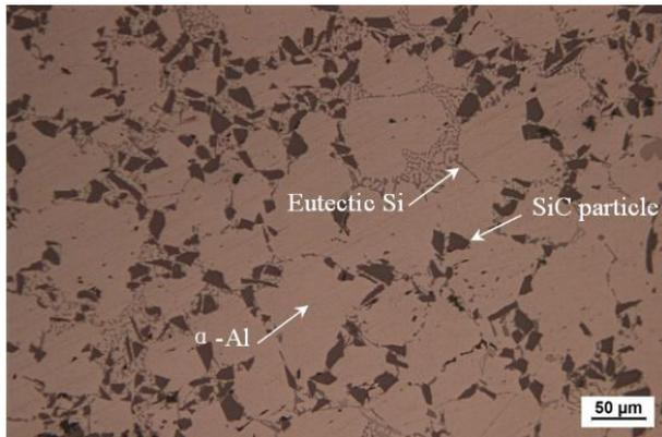
Figure 10. Microstructure of 15 vol% SiC<sub>p</sub>/Al-MMCs.
