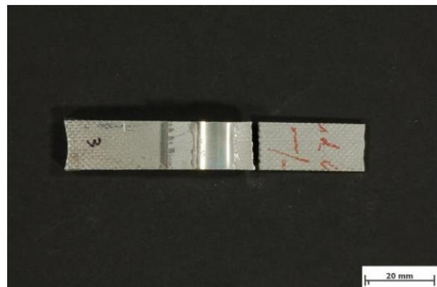
Figure 8. The tensile test result of SiC<sub>p</sub>/Al MMCs joint.
