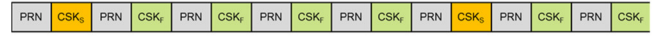
Fig. 2. Scheme for the insertion of slow and fast bursts in the PRN sequence.
