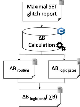
Fig 5. The automated flow for the computation of the broadening coefficient for each logic path.
