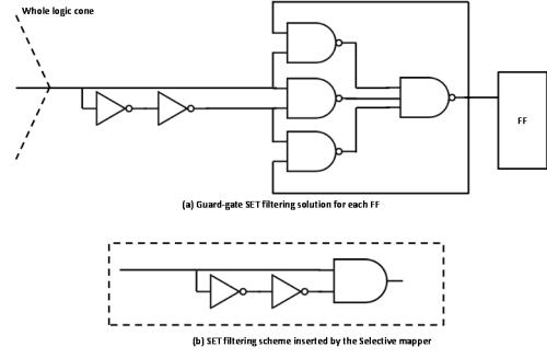
Fig 4. The GG schema for filtering SET at the input of a Flip-Flop (a) and in any position of the circuit (b).
