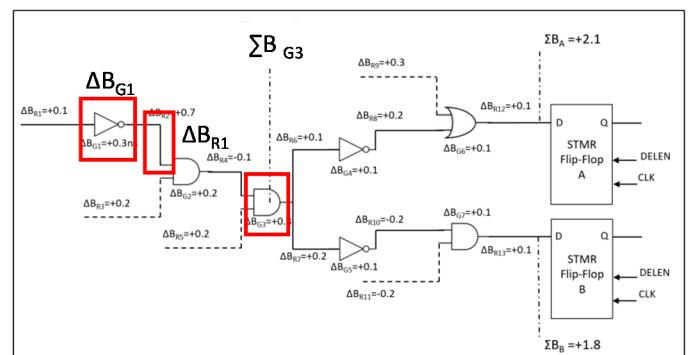
Fig 6. Identification of gate and routing considered for guard-gate insertion.
