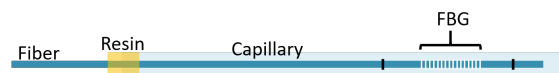
Figure 1: A schematic representation of the fiber with the FBG, inserted in a glass capillary and fixed on one side with epoxy resin.
