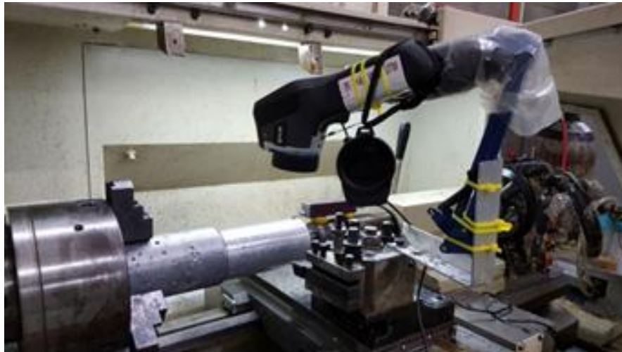
Figure 1. FLIR thermal camera mounted on turning machine tool post DWT Decomposition model
