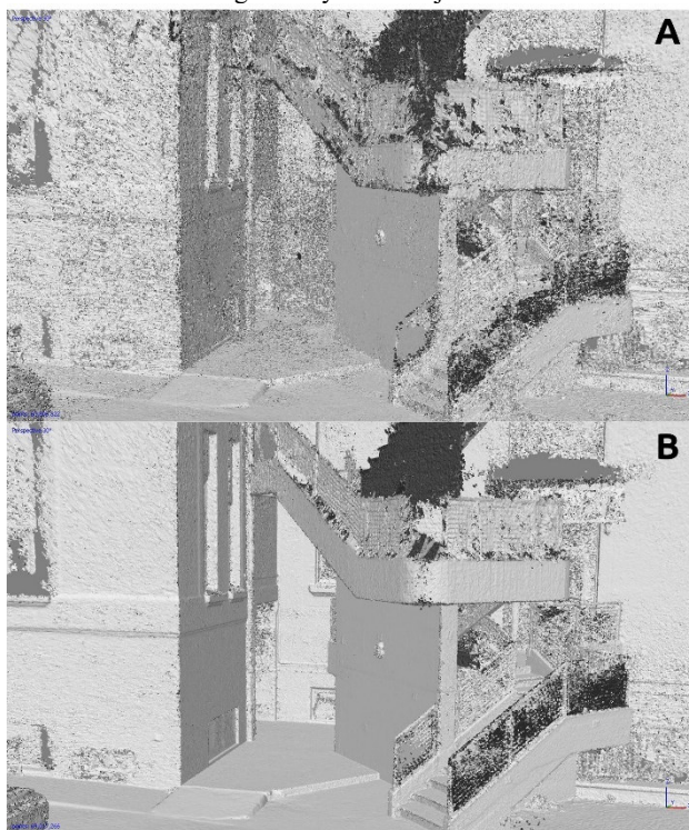
Figure 11. Visual inspection of the Dense Cloud generated in Photoscan. 360 configuration: automatic process with native Exif (A), process with modified Exif (B).
