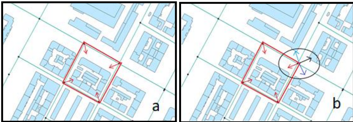
Figure 5. (a) Water demand q_{i,w} for the mesh element w , (b) water demand for the i -node.
