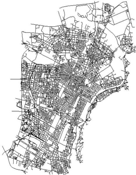
Figure 3. Global view of the water network: 19604 pipes.
