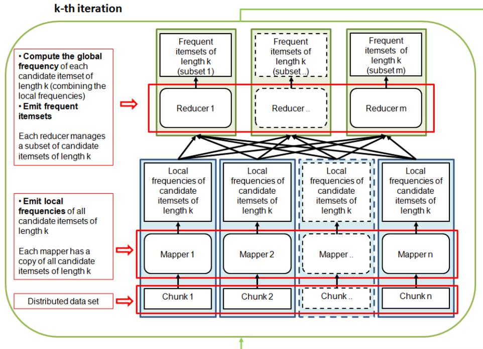
Fig. 2.3 Itemset mining parallelization: Iterative Data split approach
