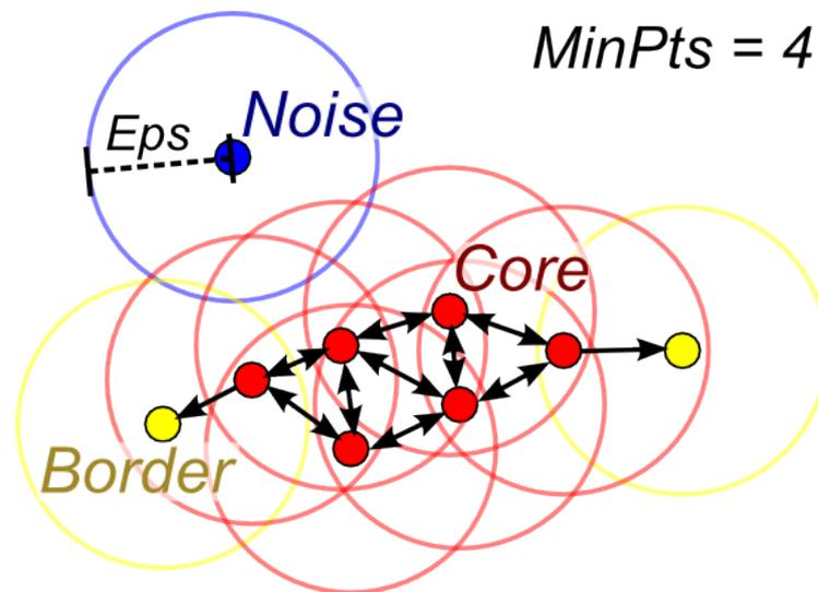
Fig. 3.2 Toy example for DBScan, with *MinPoints* set to 4. The picture highlights the area of radius *Epsilon* around each point, which can divide in *core points*, in red, *border points*, in yellow, and *noise*, in blue. Adapted from [66].
