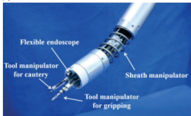
Figure 20: Master–slave robotic system introduced by Fujie et al.
