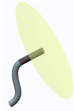
Figure 44: The darkest point at the tip represents the rigid and non-flexible endoscope cap. The yellow cone is instead the field of vision.
