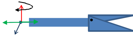
Figure 62: Scheme of gripper arm with pitch at the base and sliding (green arrows)
