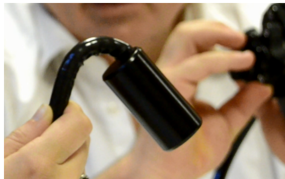
Figure 57: Flexibility test with cap 26mm diameter and 50mm length.
