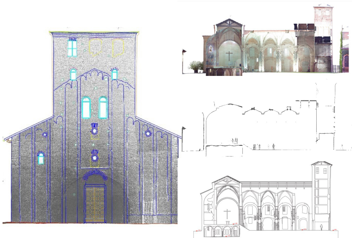
Fig. 4 – Elevation (left) and section vector-based extraction (right – Top: point cloud – Middle: section line – Bottom: complete section vector-dataset)
