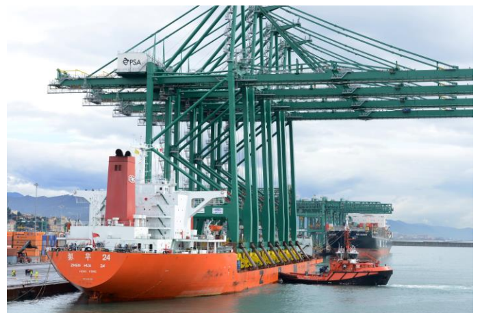
Figure 3. VTE's quay gantry cranes - gooseneck type
