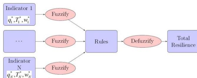
Figure 8. Full PEOPLES approach general hierarchical scheme with the weighting process included in the fuzzy system as a separate variable.
