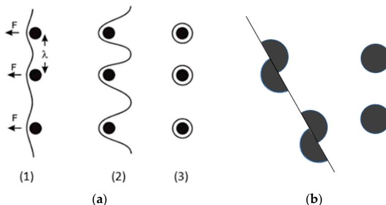
**Figure 4.** Schematic of (a) Orowan looping, (b) shearing the particles after the interaction by dislocations [100].
