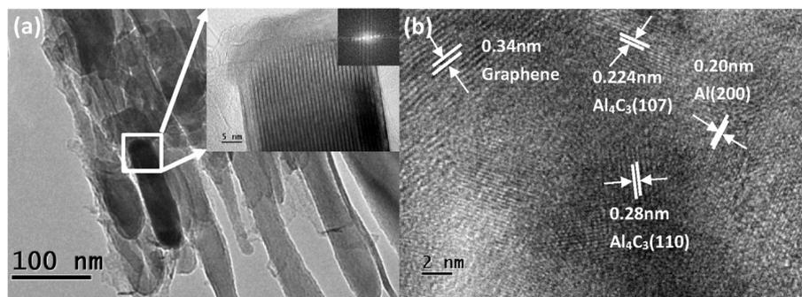
**Figure 5.** Transmission electron microscopy (TEM) and high-resolution transmission electron microscopy (HRTEM) images of Al/GNPs composites: (a) TEM image shows rod aluminum carbide with corresponding selected area diffraction (SAED) patterns, (b) graphene, Al, aluminum carbide area and their interface [121], Reproduced from [121], with permission from Elsevier, 2018.
