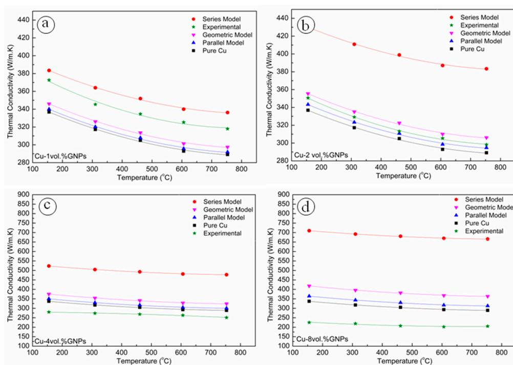
**Figure 14.** Comparison of experimental thermal conductivities of (a) Cu-1 vol % GNPs, (b) Cu-2 vol % GNPs, (c) Cu-4 vol % GNPs, (d) Cu-8 vol % GNPs, to the prediction by different models [142], Reproduced from [142], with permission from Springer Nature, 2018.
