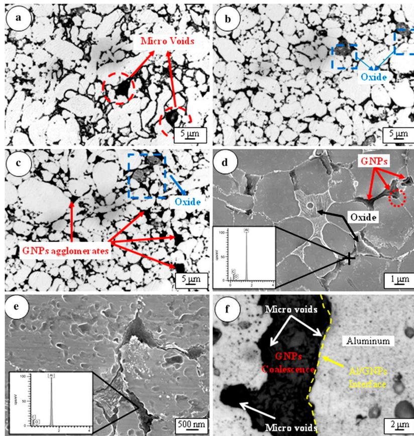
**Figure 9.** Optical microscopy (OM) micrograph of press-sintered (a) pure Al, (b) Al-0.5 wt % GNPs, (c) Al-1.0 wt % GNPs, (d) scanning electron microscopy (SEM) image of Al-1.0 wt % GNPs, (e) EDS analysis at a grain boundary, (f) a representative grain boundary of Al-1.0 wt % GNPs after sintering [131], Reproduced from [131], with permission from Springer Nature, 2017.
