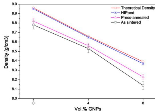
**Figure 17.** Theoretical and measured densities of composites after sintering and two different post-processing techniques (repressing followed by annealing and HIPing) [10], Reproduced from [10], with permission from Springer Nature, 2018.
