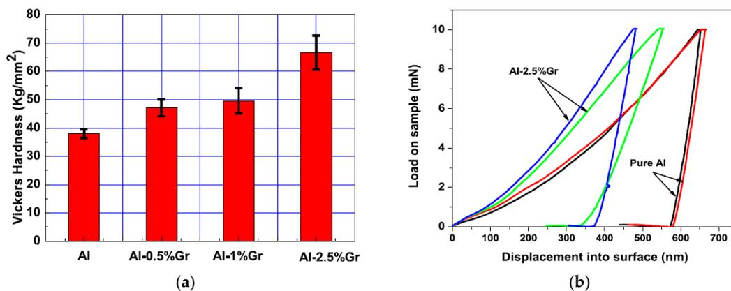
**Figure 6.** (a) The Vickers hardness and (b) load-displacement depth of nanomechanical tests of Al/GNPs nanocomposites produced by SLM [121], Reproduced from [121], with permission from Elsevier, 2018.
