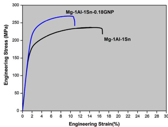
**Figure 20.** Tensile test of Mg-1Al-1Sn and Mg-1Al-1Sn-0.18GNP composites [1], Reproduced from [1], with permission from Elsevier, 2014.
