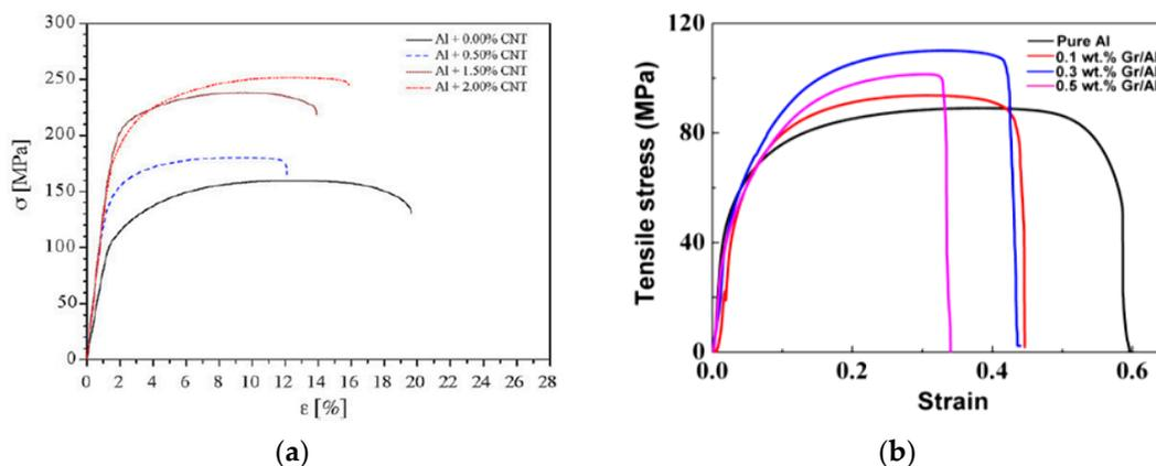
**Figure 3.** Tensile stress-strain curves of Al nanocomposites reinforced by (a) Carbon Nanotubes (CNTs)[96], (b) graphene [24], Reproduced from [96] and [24], with permission from Elsevier, 2009 and 2016.
