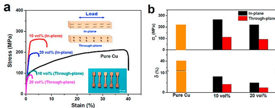
**Figure 16.** (a) Tensile stress-strain curves and (b) obtained properties of tensile strength ( $\sigma_b$ ) and elongation ( $\delta$ ) for pure Cu and 10 vol %/20 vol % GNP/Cu composites with the load parallel and perpendicular to the alignment direction [144], Reproduced from [144], with permission from Elsevier, 2018.
