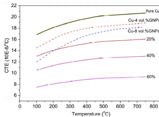
**Figure 15.** The theoretical predictions and experimental coefficient of thermal expansion of pure copper, Cu-4 vol % GNPs, and Cu-8 vol % GNPs as a function of temperature [142], Reproduced from [142], with permission from Springer Nature, 2018.
