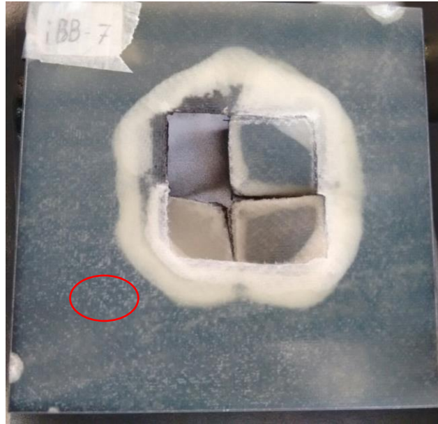
Figure 7: Micro-porosity inside a specimen
