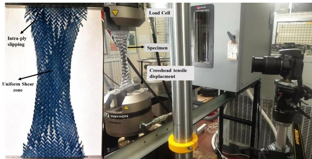
**Figure 30 a) Sample specimen shear force distribution, b) Bias extension test setup**
