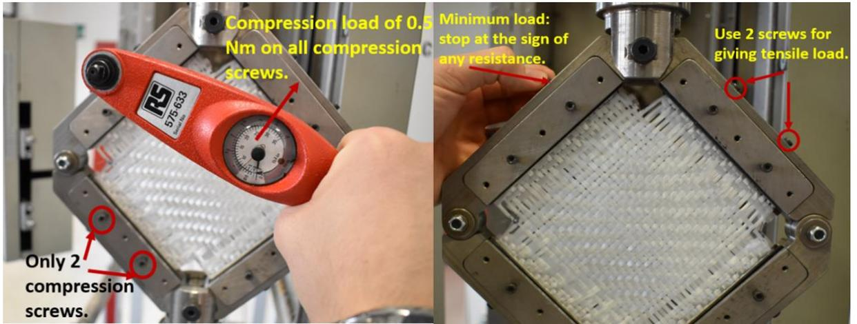
Figure 37 Trellis Frame specimen setup for good results
