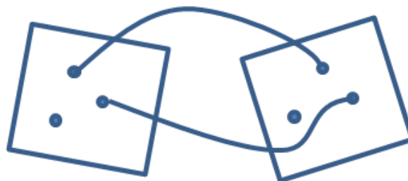
Figure 4. MicMac perform a check a-posteriori, verifying that the neighbours of a point in one image are also its neighbours in the other.
