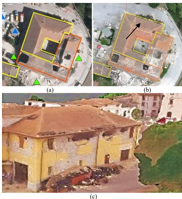
Figure 11. BDA on Accumoli site, in a sample building. The aerial image of Copernicus (a), the UAVs orthophoto (b) and a view of the considered damaged façade in the 3D model inspection (c).
