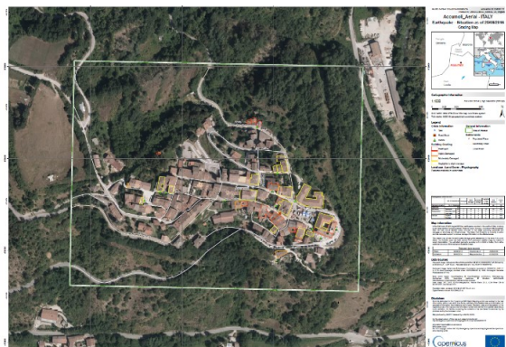
Figure 1. Post-event Grading Map for Accumoli (RI), Italy. Aerial image from © European Commission (acquired on 25/08/2016, GSD 0.1m, 0% cloud coverage) provided under COPERNICUS by CGR, Compagnia Generale Riprese aeree .
