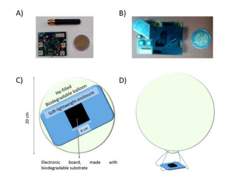
Figure 1 A) Early prototype electronic board. B) Example of the OPC (Rorato et al. Wireless Sensor Network 2013). Possible probe designs: C) ultra-lightweight model in which the electronics are comfortably placed into the He-inflated balloon and D) advanced radiosonde where the electronics hang from the balloon.
